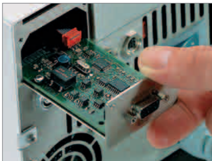
Easy replacement of interface modules
