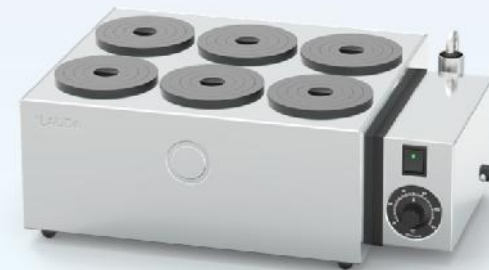
H 11 V vaporization water bath
