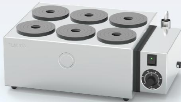
H 11 V vaporization water bath
