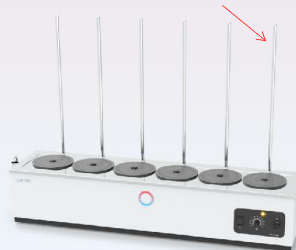
H 9 V vaporization water bath
